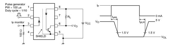
Fig. 12.1.1 Switching Time Test Circuit and Waveform
