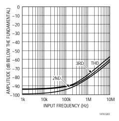
Figure 4. Distortion vs Input Frequency
