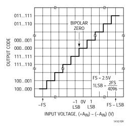
Figure 9. LTC1410 Transfer Characteristics
