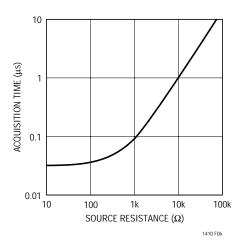
Figure 6. Acquisition Time vs Source Resistance
