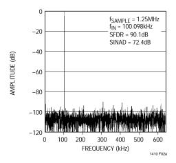
Figure 2a. LTC1410 Nonaveraged 4096 Point FFT, 100kHz Input
