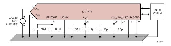
Figure 11. Power Supply Grounding Practice
