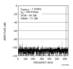
Figure 2b. LTC1410 Nonaveraged 4096 Point FFT, 600kHz Input
