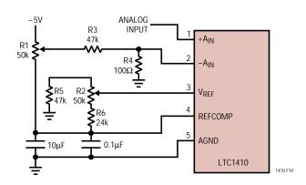
Figure 10. Offset and Full-Scale Adjust Circuit
