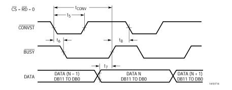
Figure 14. Mode 1a. CONVST Starts a Conversion. Data Outputs Always Enabled (CONVST = \_\_\_\_\_\_)
