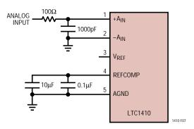
Figure 7. RC Input Filter
