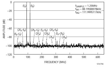
Figure 5. Intermodulation Distortion Plot
