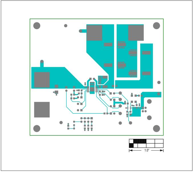
MAX17561 EV Kit PCB Layout—Component Side
