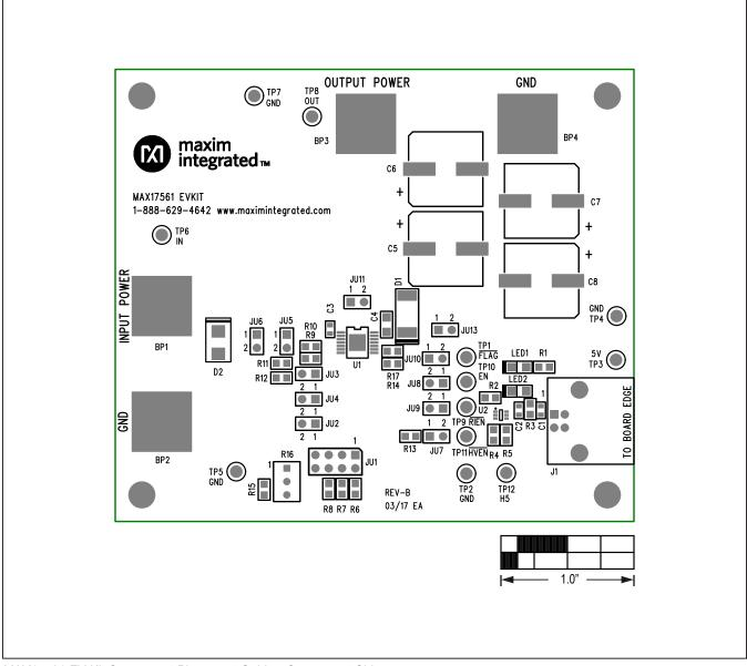
MAX17561 EV Kit Component Placement Guide—Component Side
