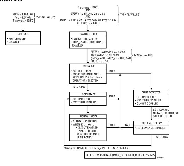
Figure 2. Start-Up and Fault Sequence
