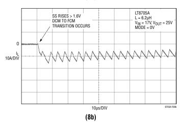
Figure 8. LT8705 and LT8705A Inductor Current During DCM to FCM Transition
