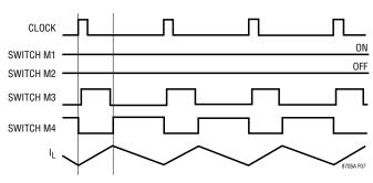
Figure 7. Boost Region (V<sub>IN</sub> << V<sub>OUT</sub>)
