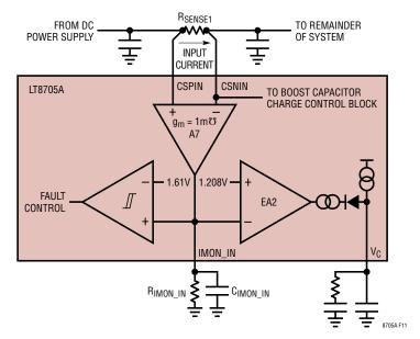
Figure 11. Input Current Monitor and Limit
