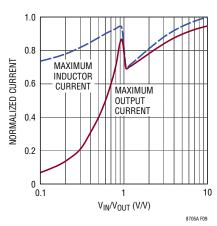
Figure 9. Currents vs V<sub>IN</sub>/V<sub>OUT</sub> Ratio
