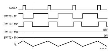
Figure 5. Buck Region (V<sub>IN</sub> >> V<sub>OUT</sub>)
