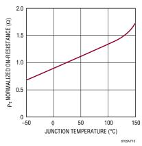
Figure 10. Normalized MOSFET R<sub>DS(ON)</sub> vs Temperature
