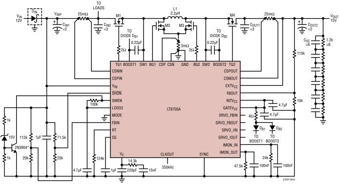
$C_{IN1},\,C_{OUT2};\,100\mu\text{F}$  20V SANYO OS-CON 205A100M  $C_{IN2},\,C_{OUT1};\,22\mu\text{F},\,25V,\,TDK$  C4532X741E226M  $C_{SC};\,60\text{F},\,2.5V$  COOPER BUSSMAN HB1840-2R5606-R
