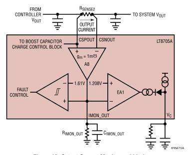
Figure 12. Output Current Monitor and Limit
