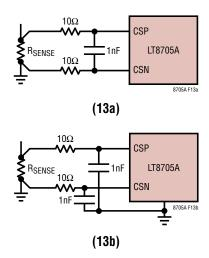
Figure 13. Inductor Current Sense Filter
