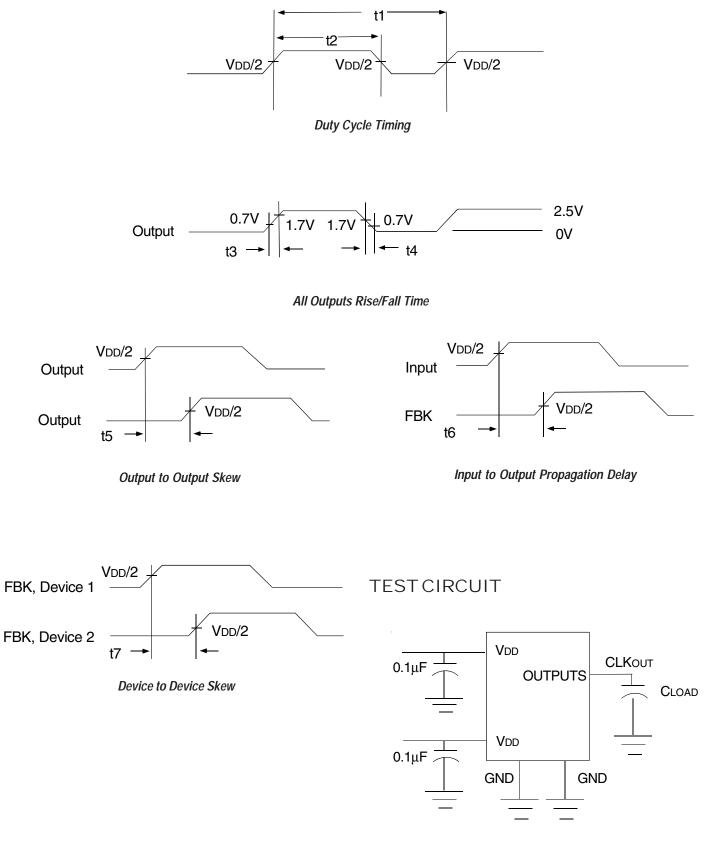
Test Circuit for all Parameters
