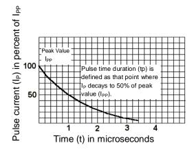
FIG. 2 Pulse wave form for exponential surge for 10/1000 µs
