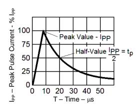
FIGURE 3 8/20  $\mu s$  CURRENT IMPULSE WAVEFORM TEST WAVEFORM PARAMETERS:  $t_r = 8 \mu sec$   $t_p = 20 \mu sec$
