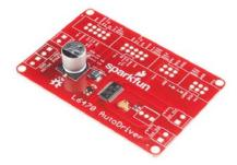
The AutoDriver board is based on the STMicro L6470 dSPIN stepper motor driver. This powerful chip allows you to control a stepper motor with a voltage from 8-45V at 3A<sub>rms</sub> over an SPI connection. Compared to traditional step/direction motor controllers, it offers a number of advantages:
