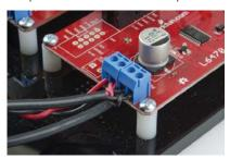
It's generally a good idea to hook up the power to the RedBoard and logic circuitry before you power the AutoDrivers; do note that you can't access the AutoDriver boards via SPI until BOTH parts are powered, however.
