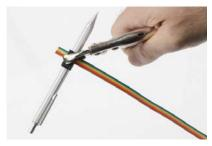
Next, we'll want to crimp on one of the other connectors. See the image below for proper orientation; crimping this in place is much easier because it doesn't have pins to be damaged.
