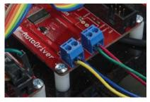
The above picture shows the order I've selected for our medium stepper motors. It's probably a good idea to use the same wire order on both boards, so the relative direction of both motors is the same. If you need the direction to be opposite for the two motors (say, to drive the wheels of a robot), you can simply reverse the order of one pair of wires.
