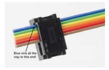
Before you apply pressure to crimp the connector closed, you need something to prevent the pins from being smashed in the process. A pencil fits between the pins perfectly.
