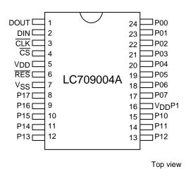
MFP24S (300mil): lead-free type/MFP24SJ (300mil): lead-free type
