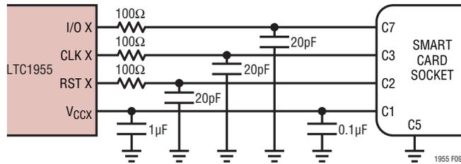
Figure 8. Additional Components for Improved Compliance Testing
