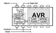
The FS2009(AVR-JTAG) supports programming of the Atmel ATmega AVR Microcontroller Family using the JTAG algorithm. This allows the FS2009 to program the ATmega devices at high speed via the JTAG port of the Target Device.
