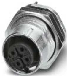
Sensor/actuator flush-type socket, 5-pos., M12 SPEEDCON, shielded, A-coded, rear/screw mounting with Pg9 thread, with straight solder connection
