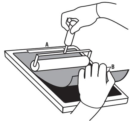
Relax film slightly allowing tab 'A' edge to come close to LCD panel, but not touch. With free hand, use roller to laminate film into place in one continuous sweep. Remove tabs 'A' and 'B'. Use plastic stylus to complete lamination along edges as necessary. Clean with acetone as necessary.
