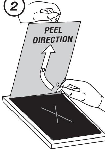
Raise DQC film and liner by gently lifting up tab 'B'. Use caution to grab tab only, not the film. Raise film high enough to allow liner to be removed. Grip tab 'C' firmly with free hand and gently pull in direction of arrow 'D' to separate liner from DQC adhesive. Pull slowly and gently to advance separation of liner along tab 'A' edge, before pulling toward tab 'B' edge.
