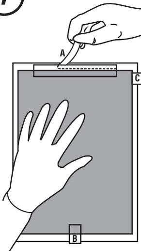
Place film, liner side down, onto LCD panel, and center within metal bezel. Holding film firmly in place with one hand, remove liner from tab 'A' and adhere tab A to metal bezel. Check film alignment; realign if necessary. Then place tab 'B', Scotch® Brand Tape on the top surface of the film.
