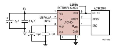
LTC1404 Interface to the ADSP2181's SPORTO (Frame Sync is Generated from RFS0)
