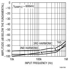
Figure 4. Distortion vs Input Frequency in Bipolar Mode
