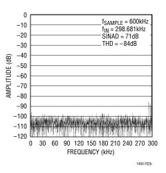
Figure 2b. LTC1404 Nonaveraged, 4096 Point FFT Plot with 300kHz Input Frequency in Bipolar Mode
