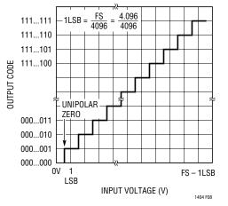
Figure 8. LTC1404 Unipolar Transfer Characteristics
