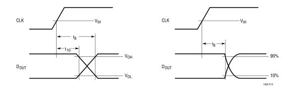
Figure 14. CLK to D<sub>OUT</sub> Delay
