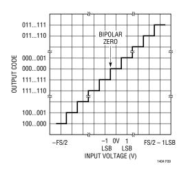
Figure 9. LTC1404 Bipolar Transfer Characteristics
