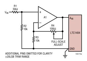
Figure 10a. LTC1404 Full-Scale Adjust Circuit
