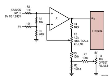
Figure 10b. LTC1404 Offset and Full-Scale Adjust Circuit
