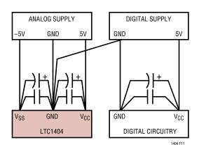
Figure 11. Power Supply Connection
