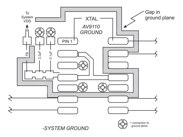
This is the recommended layout for the AV9110 to maximize clock performance. Shown are the power and ground connections, the ground plane, and the input/output traces.
