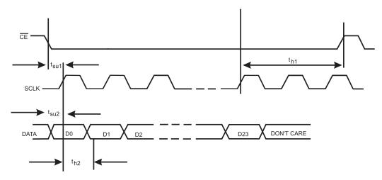
Figure 1 - Serial Programming
