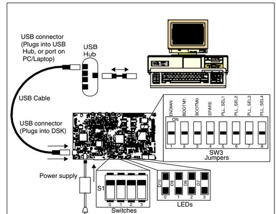
6. Make sure your DSK CD-ROM is installed in your CD-ROM drive. Now connect the DSK to your PC using the included USB. After few seconds Windows will launch its "Add New Hardware Wizard" and prompt for the location of the DSK drivers.
