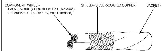
JACKET - RADIATION-CROSSLINKED, MODIFIED CONDUCTIVE ETFE COLOR - BLACK
