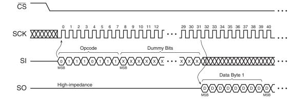
Figure 25-9. Status Register Read (Opcode D7h)
