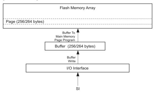
Figure 23-2. Buffer Write
