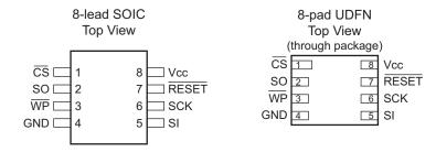
Note: 1. The metal pad on the bottom of the UDFN package is not internally connected to a voltage potential. This pad can be a "no connect" or connected to GND.
