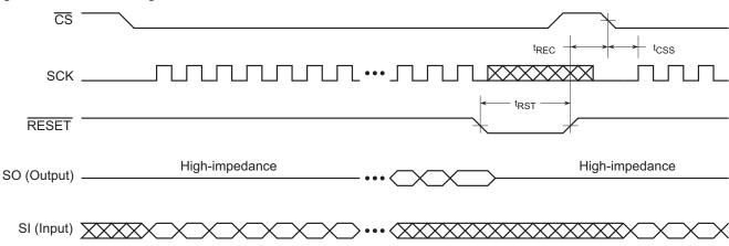
Note: 1. The  $\overline{\text{CS}}$  signal should be in the high state before the  $\overline{\text{RESET}}$  signal is deasserted.
