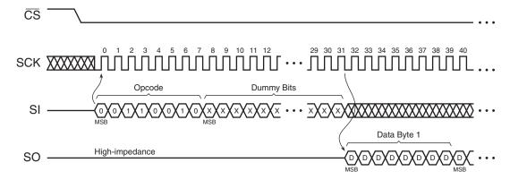
Figure 25-8. Read Security Register (Opcode 77h)
