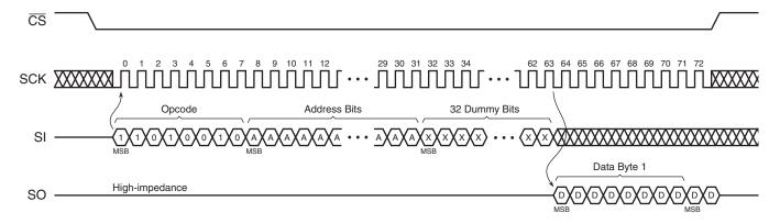
Figure 25-5. Buffer Read (Opcode D4h)
