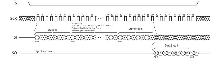
Figure 25-6. Buffer Read – Low Frequency (Opcode D1h)
