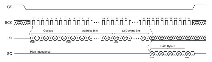
Figure 25-2. Continuous Array Read (Opcode 0Bh)
