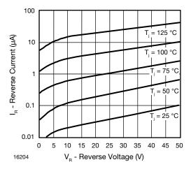
Fig. 1 - Reverse Current vs. Reverse Voltage
