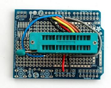
Follow the protoshield tutorial to solder in the Red LED into **LED1** position, Green LED into **LED2** position. Also solder in the two 1.0K resistors next to the LEDs. We'll use the LEDs as
