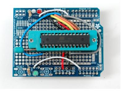
Next add **S1**switch which you will press to start the programming process. You can just solder a wire (yellow) from the breakout near **S1** to **Analog 1**.
