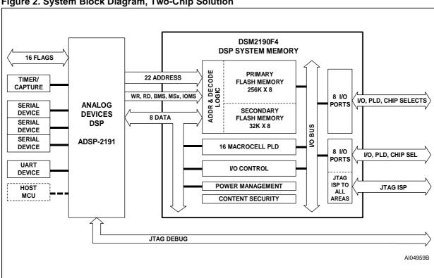
Figure 2. System Block Diagram, Two-Chip Solution
