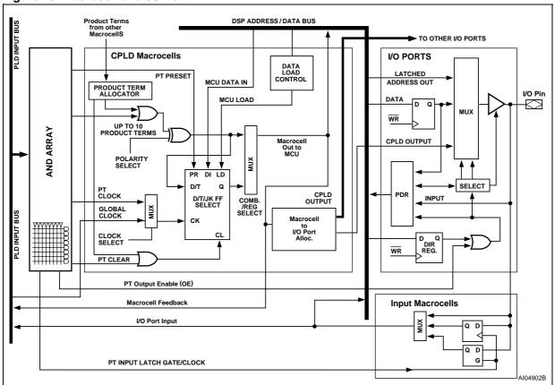
Output Macrocell (OMC). Eight of the Output Macrocells (OMC) are connected to Port B pins and are named as McellAB0-McellAB7. The other eight Macrocells are connected to Ports B or C pins and are named as McellBC0-McellBC7. OMCs may be used for internal feedback only (buried registers), or their outputs may be routed to external Port pins.
