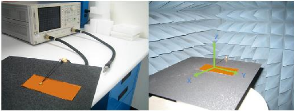
Figure 1. Impedance measurements (left hand) and peak gain, average gain, efficiency and radiation pattern measurements (right hand).
