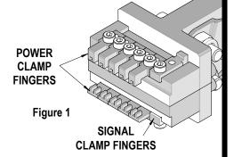
For the clamp fingers that clamp the power bay, note that the front and rear clamps are different. The signal bay clamp fingers always engage the middle rectangular hole above the signal bay.
