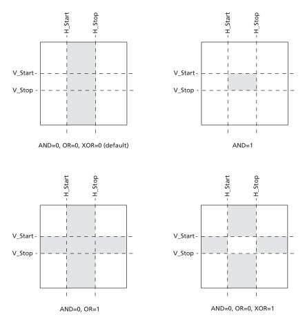
Shading indicates when USER\_x signal is active
