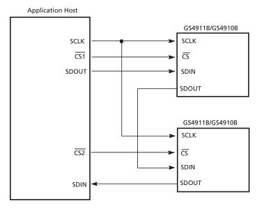
Figure 3-14: GSPI Application Interface Connection
