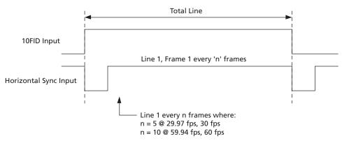
Figure 3-5: 10FID Input Timing
