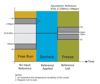
Figure 3-2: Output Accuracy and Modes of Operation
