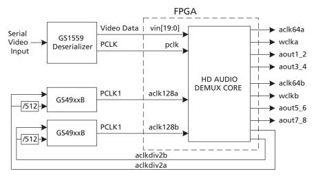
Figure 3-13: Audio Clock Block Diagram for HD Demux Operation
