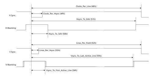
Figure 3-12: Custom Timing Parameters
