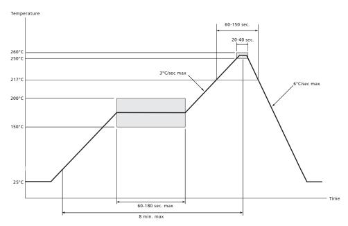
Figure 6-1: Maximum Pb-free Solder Reflow Profile (preferred)
