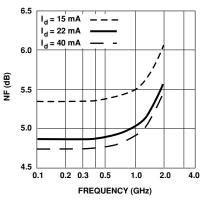
Figure 5. Noise Figure vs. Frequency.
