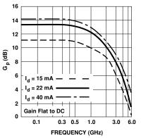
Figure 1. Typical Power Gain vs. Frequency.
