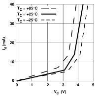
Figure 2. Device Current vs. Voltage.
