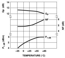
Figure 3. Output Power at 1 dB Gain Compression, NF and Power Gain vs. Case Temperature, f = 1.0 GHz,  $I_d$  = 22 mA.
