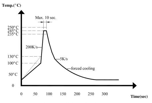
Recommendable wave soldering condition is as follows.
