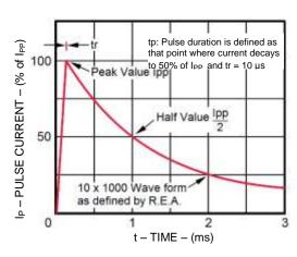
FIGURE 1 Pulse Waveform for 10/1000 µs that point where the pulse current
