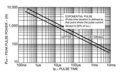
FIGURE 2 Peak Pulse Power vs. Pulse Duration
