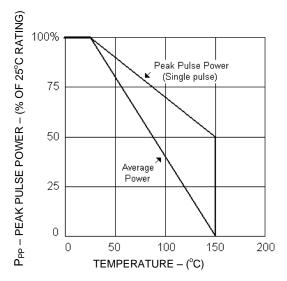
FIGURE 3 **Derating Curve**
