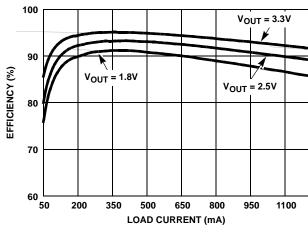
FIGURE 1. EFFICIENCY vs LOAD CURRENT (VIN = 5.0V)
