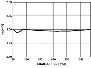
FIGURE 2.  $V_{OUT}$  vs LOAD CURRENT ( $V_{IN}$  = 5V)
