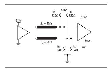
Figure 3B. 3.3V LVPECL Output Termination
