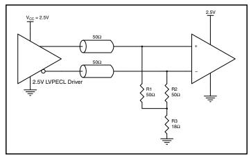
Figure 4B. 2.5V LVPECL Driver Termination Example
