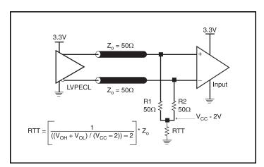
Figure 3A. 3.3V LVPECL Output Termination
