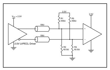
Figure 4A. 2.5V LVPECL Driver Termination Example
