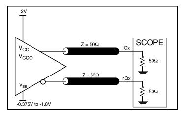
**LVPECL Output Load AC Test Circuit**
