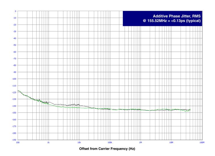
As with most timing specifications, phase noise measurements has issues relating to the limitations of the equipment. Often the noise floor of the equipment is higher than the noise floor of the device. This
