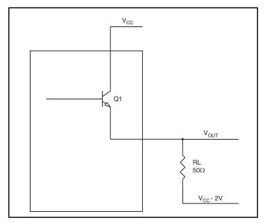
Figure 5. LVPECL Driver Circuit and Termination
