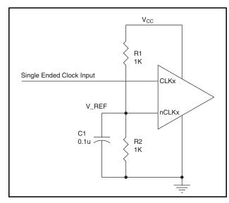
Figure 1. Single-Ended Signal Driving Differential Input
