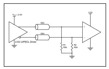
Figure 4C. 2.5V LVPECL Driver Termination Example
