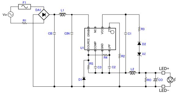
Figure 1. Application Circuit
