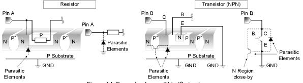
Figure 14. Example of monolithic IC structure
