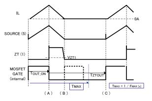
Figure 13. Maximum Frequency Operation
