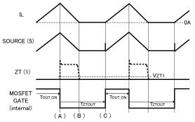
Figure 12. ZT Trigger Timeout Operation
