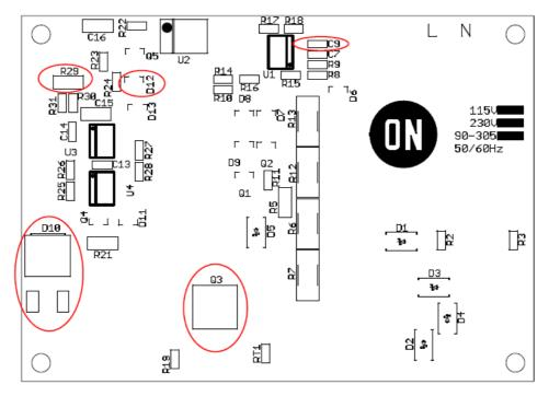
Figure 4. Bottom Side PCB Component Locations
