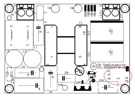
Figure 5. PCB Holes for Transformer Leads
