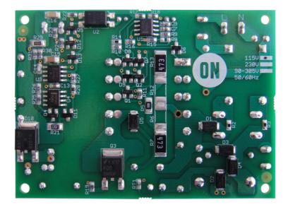
Figure 2. Bottom Side of Board
