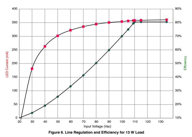
Efficiency performance is shown in Figure 6 as well. Note the efficiency remains above 70% until the output current drops to about 70 mA. The output voltage is about 34 V meaning the delivered power is about 2.4 W or less than 20% of the full power. As the current delivered is reduced, the fixed losses for startup and biasing begin to dominate the efficiency curve resulting in a steep drop off of efficiency.
