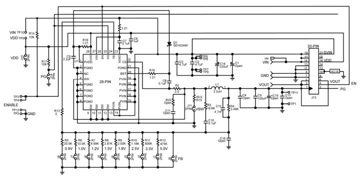
Schematic of MIC26601 Evaluation Board (J11, R13, R15 are for testing purposes)
