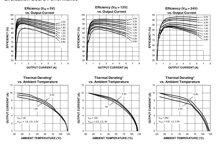
**Die Temperature\***: The temperature measurement was taken at the hottest point on the MIC26601 case mounted on a 5 square inch 4 layer, 0.62", FR-4 PCB with 2oz finish copper weight per layer, see Thermal Measurement section. Actual results will depend upon the size of the PCB, ambient temperature and proximity to other heat emitting components.
