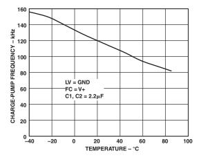
TPC 13. Charge-Pump Frequency vs. Temperature
