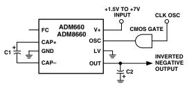
Figure 7. ADM660/ADM8660 External Oscillator
