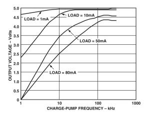
TPC 7. Output Voltage vs. Charge-Pump Frequency
