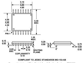
Figure 12. 16-Lead Thin Shrink Small Outline Package [TSSOP] (RU-16) Dimensions shown in millimeters
