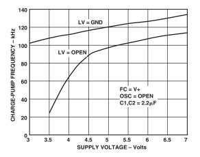
TPC 12. Charge-Pump Frequency vs. Supply Voltage
