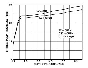
TPC 9. Charge-Pump Frequency vs. Supply Voltage
