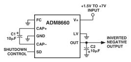
Voltage Inverter Configuration with Shutdown (ADM8660)
