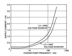
TPC 5. Power Supply Current vs. Charge-Pump Frequency
