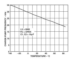
TPC 10. Charge-Pump Frequency vs. Temperature
