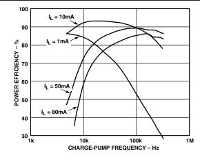
TPC 4. Efficiency vs. Charge-Pump Frequency
