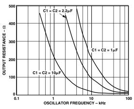
Figure 9. Output Impedance vs. Oscillator Frequency
