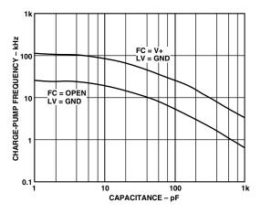
TPC 11. Charge-Pump Frequency vs. External Capacitance
